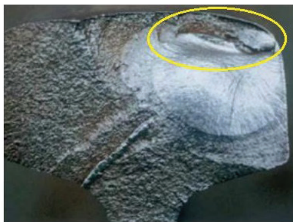
Initiation from inside the gauge corner area
