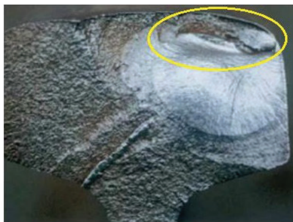
Initiation from inside the gauge corner area
